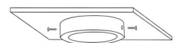
4. Installation complete After fitting the main body and the hanging plate, align the holes on the side and tighten them with screws
